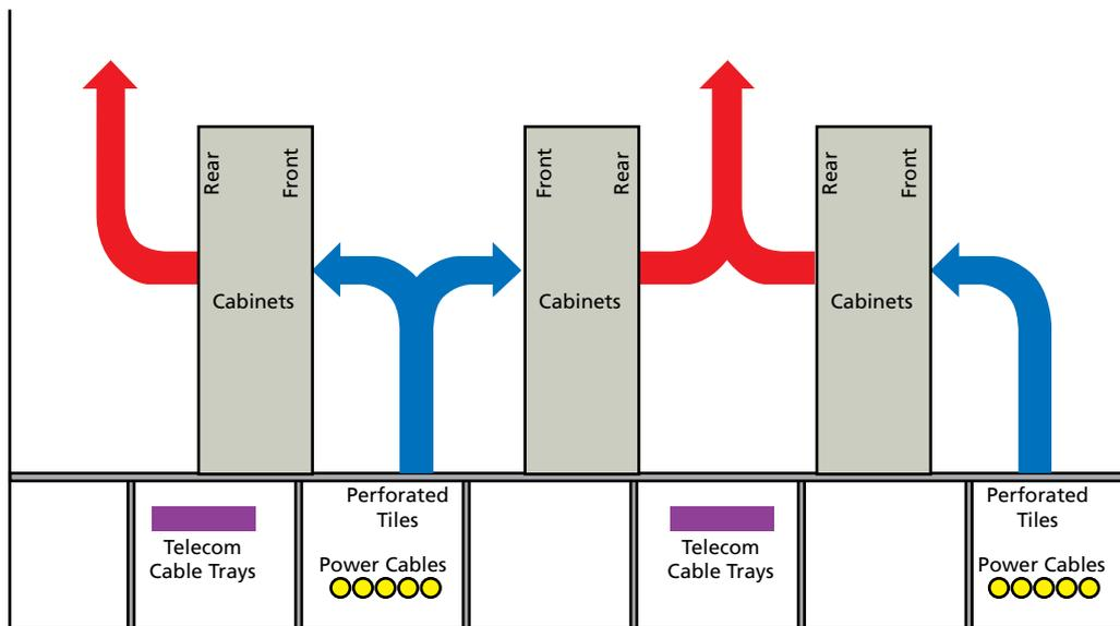
Figure 2. Hot Aisle/Cold Aisle Cooling
